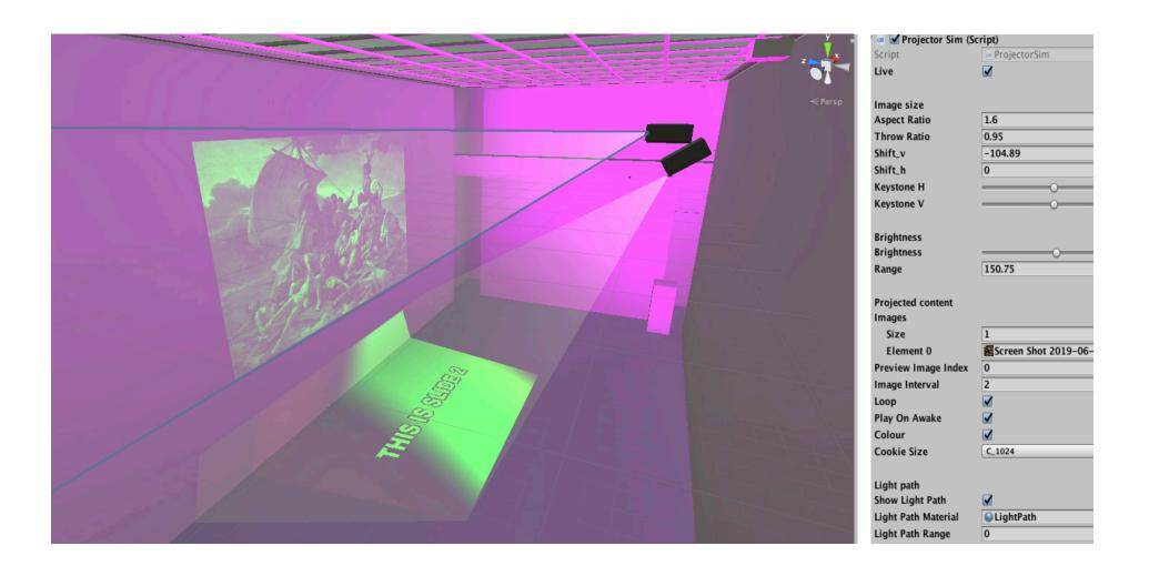
A virtual simulation is being carried out to see the layout of projectors using a projector simulator. Details and specifications of projectors are feeded into this which gives the the exact area a projector can cover from the distance. The 3D model of the room with exact dimensions were combined with this to determine estimated projector locations and issues that may arise with shadowing lighting etc.
